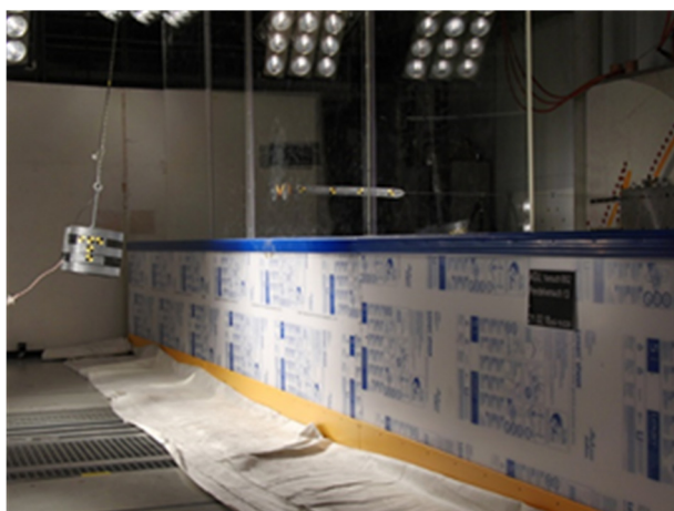
Figure 4 New impactor used to test an ice hockey board
